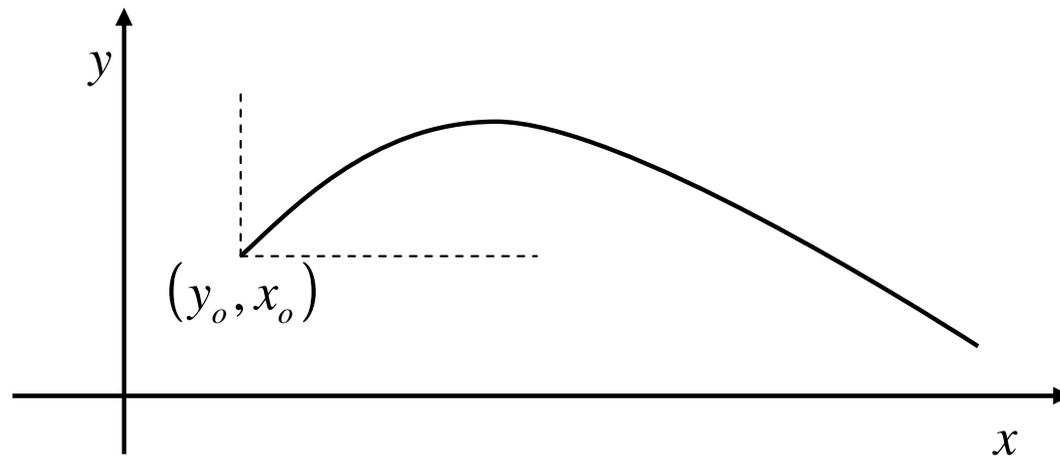
$$\vec{r} = \begin{cases} x = x_0 + v_{ox}t \\ y = y_0 + v_{oy}t - \frac{gt^2}{2} \end{cases}$$
