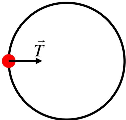
$$\begin{aligned} T &= ma_c \\ &= \frac{mv^2}{r} \end{aligned}$$
