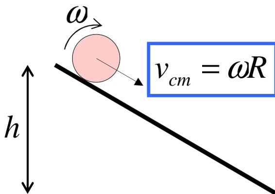
$$\left( \frac{I_{cm} \omega^2}{2} + \frac{M v_{cm}^2}{2} \right) + \Delta U_g = 0$$
