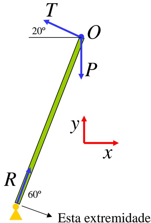
$$\begin{aligned} \text{em } x : & \left\{ -T \cos(20) + R \cos(60) = 0 \right. \\ \text{em } y : & \left\{ -P + T \sin(20) + R \sin(60) = 0 \right. \end{aligned}$$
