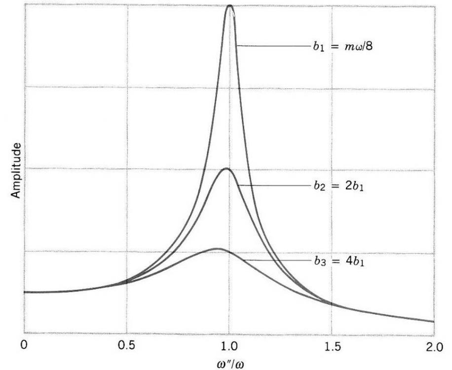
Figure 20 The amplitude  $F_m/G$  of a forced oscillator as the
