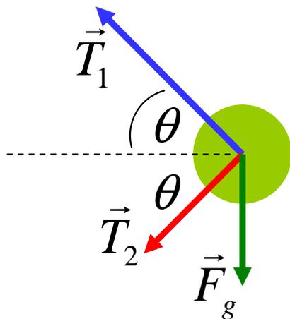
$$\begin{cases} T_1 \sin(\theta) - T_2 \sin(\theta) - mg = 0 \\ T_1 \cos(\theta) + T_2 \cos(\theta) = ma_c \end{cases}$$
