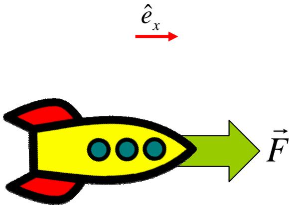
$$\begin{aligned} F &= ma \\ &= m \left( \frac{\Delta v}{\Delta t} \right) = 500 \frac{444 - 0}{1.8} \\ &= 123 \text{ kN} \end{aligned}$$
